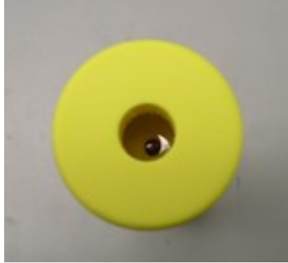
The “Pinger Operating LED” can be seen through the port at the end of the pinger.
