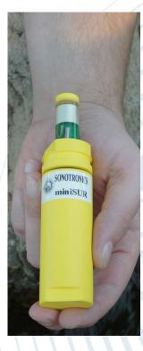
The miniSUR, <u>miniature Submersible Ultrasonic Receiver</u> provides new features to aid in passive tracking of ultrasonic tagged animals.
