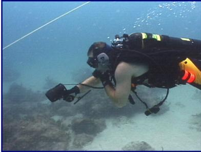
The Sonotronics Underwater Diver Receiver (UDR) allows a diver to locate and approach any object in a marine environment previously marked with a Sonotronics equipment marker transmitter (EMT), as well as other manufacturers' compatible pingers. These objects include submersibles, water monitoring equipment, divers, or virtually any other underwater object. Applications include military, ocean oil drilling operations, surveying, and fisheries..
