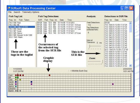
**SURsoft** data processing center is a new addition to the SURsoft software package. The DPC allows the user to instantaneously sort data from SUR output files. automatically calculate telemetry from transmitters, receive statistics about fish detections, and view a graphic display showing the activity at an SUR. The graphic results can be exported as a bitmap file and used in presentations, etc.
