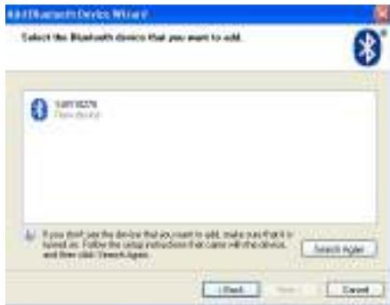
The SUR is now 'discovered', which leads to the next step, pairing. This step involves establishing a unique relationship between the host PC and the Bluetooth device, exchanging a 'passkey' to allow error free communication between these devices. Unless otherwise specified, all SUR-3BT units have a passkey of "1234", and is provided in the next step by highlighting the SUR device, clicking "Next", and filling in the subsequent screen:
