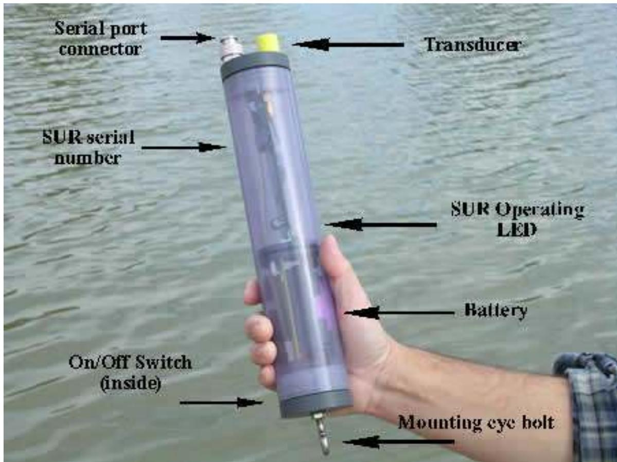
**Caution!!** Never hold the transducer or Serial Port connector when opening: use the rim of the gray cap only. (A 'grip wrench' is recommended for loosening the SUR caps.)
