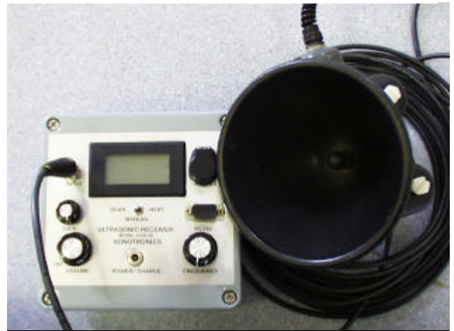
Figure 6. Sonic receiver (left) and directional hydrophone used by researchers on Lake Pend Oreille to find tagged fish and determine habitat use.
