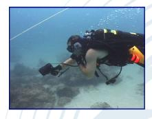
The Sonotronics Underwater Diver Receiver (UDR) allows a diver to locate and approach any object in a marine environment previously marked with a Sonotronics equipment marker transmitter (EMT), as well as other manufacturers' compatible pingers. These objects include submersibles, water monitoring equipment, divers, or virtually any other underwater object. Applications include military, ocean oil drilling operations, surveying, and fisheries...
