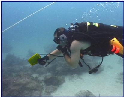
The Sonotronics Underwater Diver Receiver (UDR) allows a diver to locate and approach any object in a marine environment previously marked with a Sonotronics equipment marker transmitter (EMT), as well as other manufacturers' compatible pingers.
