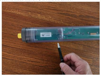
When a Bluetooth connection is made, this LED will change to a "double-blink" about once per second, switching back to a slower single blink once this connection is disabled.
