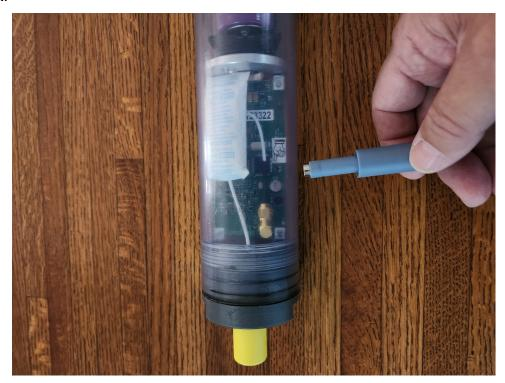
When active, the BLE activity LED will start to blink about every 3 seconds until a connection is made with a PC or Android device:
